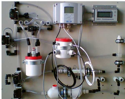
humidity test bench for sensor check
