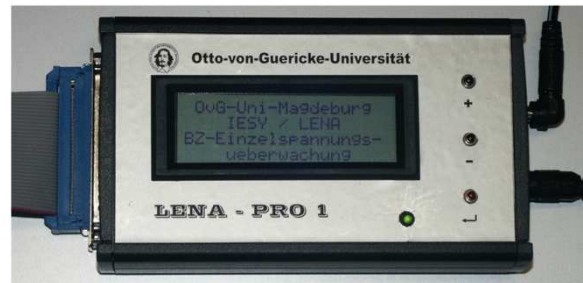
FC single cell voltage measurement device
