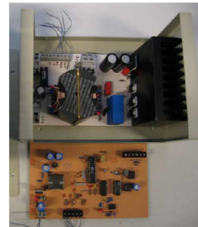
500W DC/DC converter 12-22V/24V
