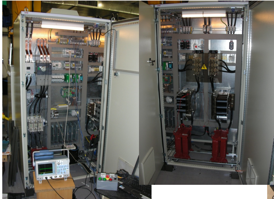
200kW plasma torch power supply
